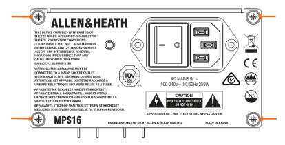
(i) dLive MixRacks ship with one PSU fitted. A second PSU can be fitted for redundancy (part number MPS-16). Loosen the 4 captive thumb screws securing the blank panel\*, slide the PSU into the slot, and tighten the 4 captive thumb screws indicated above. The MixRack will automatically switch between the supplies without interruption to the audio should one fail.
